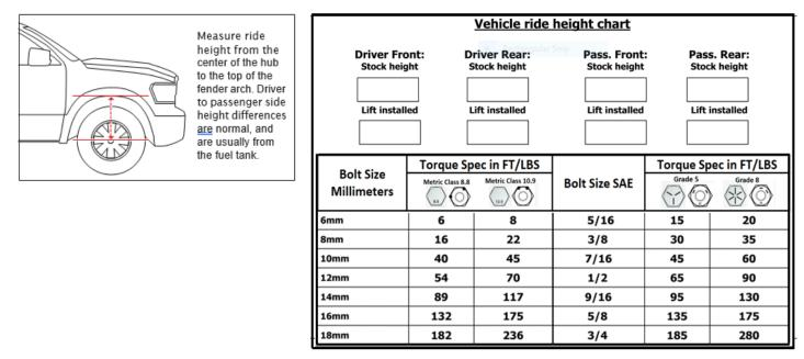
**Note:** The torque values are intended as a general guideline. Torque values for specific applications may vary. Bison Off Road does not warrant this information to be accurate and disclaims all liability for any claims or damage which may result from its use. See vehicle manufacturer's service manual for torque values.
