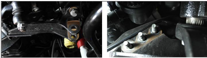
3. Install the Bison Offroad Extended Track Bar Bracket. Thread the Track Bar using the new Track Bar bolt. Installing the Track Bar may require a soft mallet or moving the steering wheel of the truck. Make sure that the Stop Cam washers are installed but are not yet captured in the bracket.
