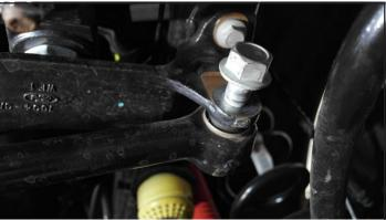
2. Remove the bolts holding the Track Bar Bracket to the frame. Keep the bolts for reuse.
