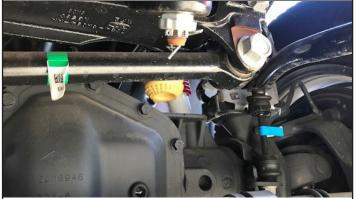
Using a large breaker bar, remove the Track Bar Rod. The OEM Track Bar bolt and nut should not be used on the new Bison Offroad Track Bar, as it is too short.
