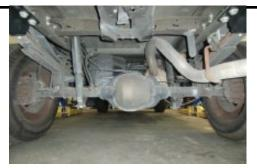
1. Place vehicle on level ground and lift and support by frame.
