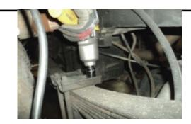
4. Remove u-bolt nuts on top of leaf spring plate
