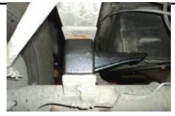
6. Remove OE axle block and replace w/ new lift block.
