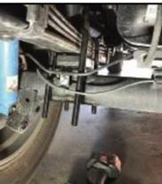
6. Replace the bottom plate and nuts with the sup-plied hardware. Review all notes in the Post Installation section.
