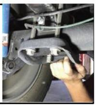
3. Lower the rear differential so there's enough room to install the block kit, and reset the jack stands.
