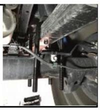
4. Install the block kit, making sure that the locating pins are lined up.
