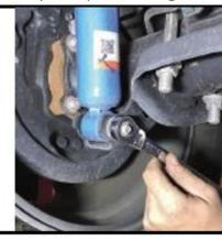
2. Disconnect the lower leaf spring brackets and remove the bracket and U bolts.
